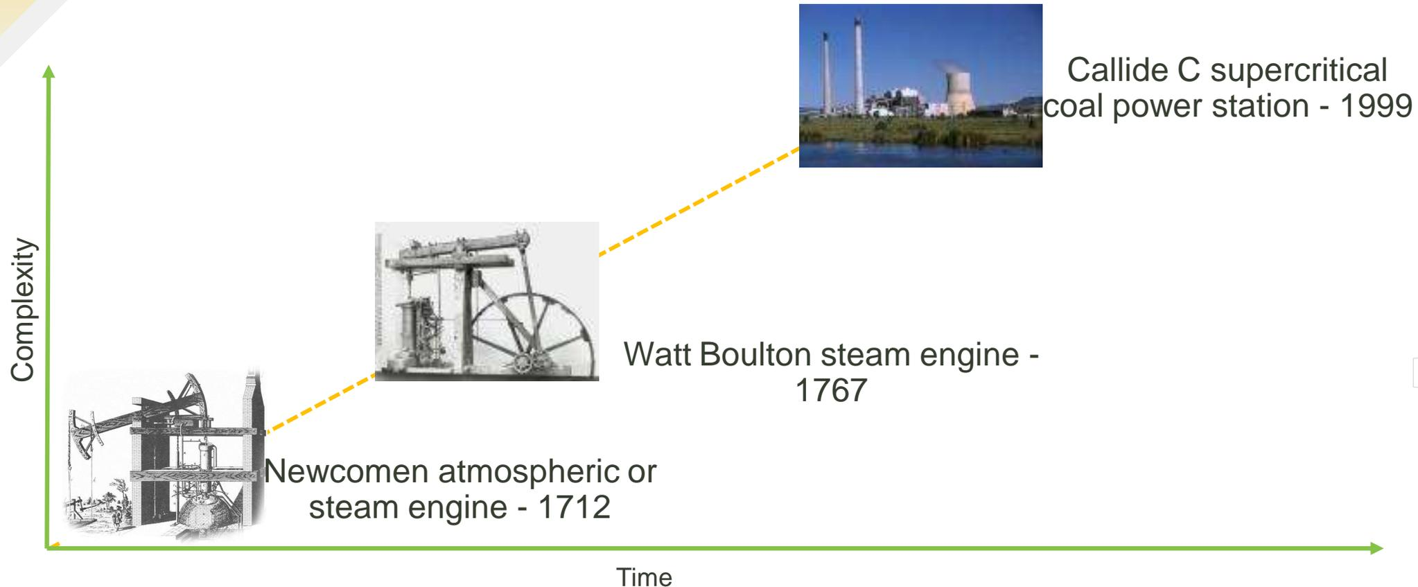
**Newcomen's atmospheric engine, originally used to dewater coal mines, was a precursor to fossil fuel usage**
